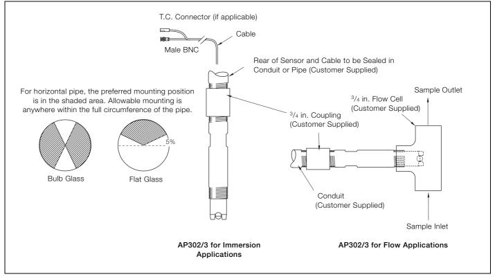
Fig. 2.3 Installing the AP302/3
