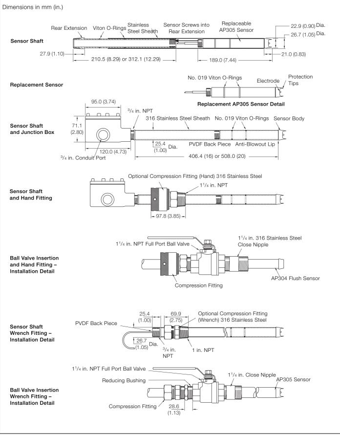
Fig. 1.5 AP304/5 Sensors and Overall Dimensions
