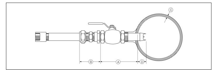
Fig. 2.5 Installing the AP304/5 – Installation Measurements
