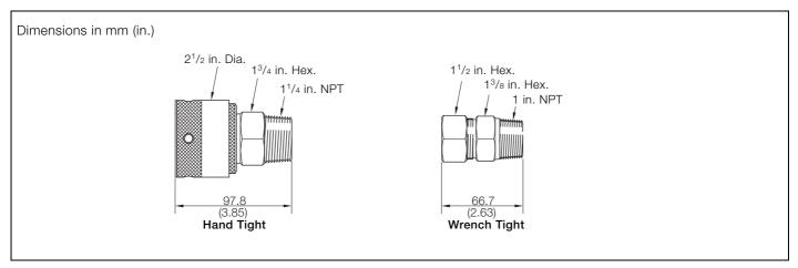
Fig. 1.4 AP304/5 Compression Fitting Dimensions
