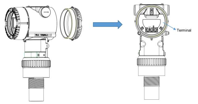
Fig. 3-1: Cable connection area
