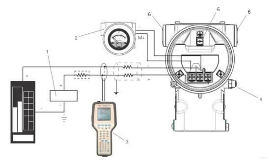
Fig. 3-2: Electrical connection - Hart version
