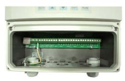
Figure 1 Terminal access on the LST400
