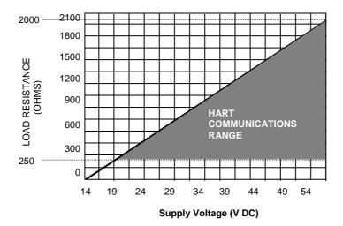
Figure 1-1 Supply Voltage Requirements, HART and Analog Versions
