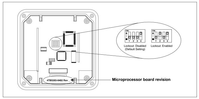
Figure 3-4 Lockout switch
