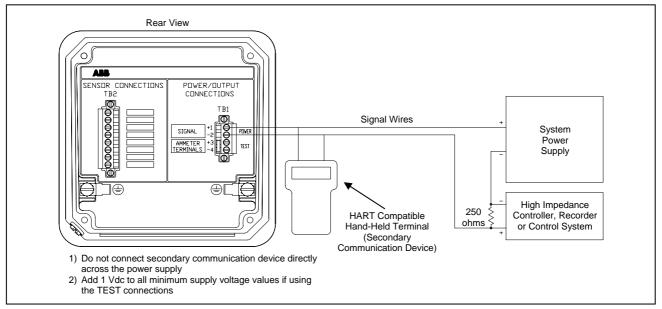
Figure 3-1 Analog Mode Wiring Diagram
