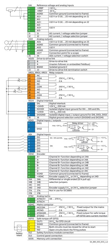
01 Control unit SDCS-CON-H01 The DCS880 single drives offers a wide range of standard interfaces. In addition the drive has three option slots that can be used for extensions including fieldbus adapter modules, input/output extension modules, feedback modules and a safety functions module.
