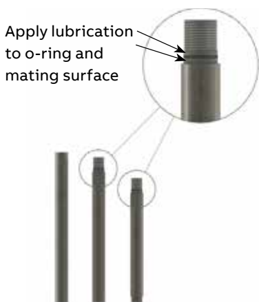
Figure 8 W7 Well Threaded Connection
