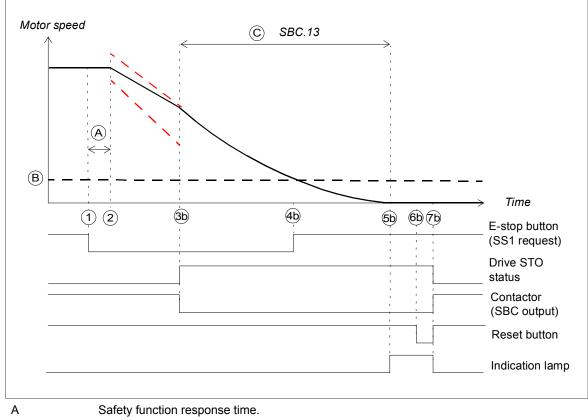
Case B: The motor speed does not follow the user-defined stop ramp monitoring window
