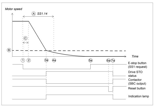
Case A: The motor speed reaches the zero speed limit within the user-defined time
