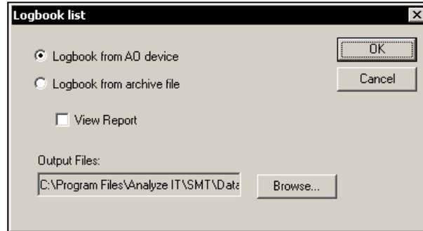
The “Logbook list” tool is used to save the contents of a gas analyzer or configuration file log as text (logbook listing); in this format it can be processed using MS Excel. Additionally, the log can be viewed on the screen.
