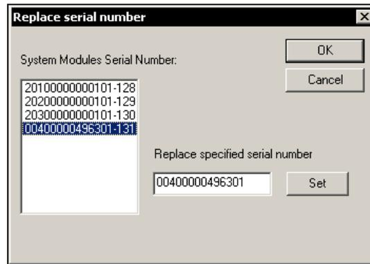
The configuration data from a gas analyzer can be transferred to a different gas analyzer using the “Replace serial number” tool.
