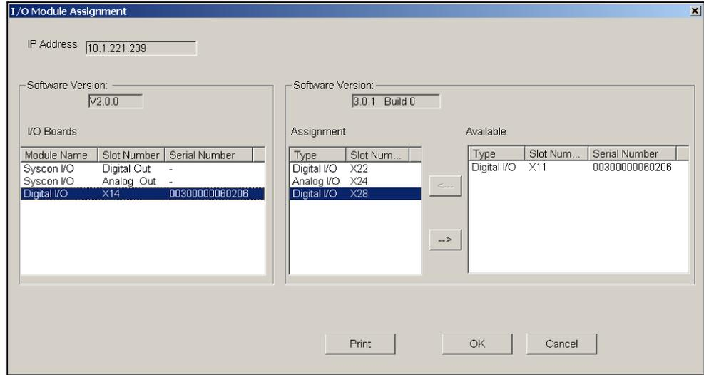
In the “I/O Boards” list (left) the Syscon I/O’s and I/O boards as in the V 2.0 configuration file saved in step 1 are displayed.
