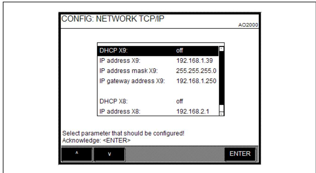
**Network Connection** Both Ethernet 10/100/1000BASE-T interfaces can be used to link the gas analyzer to an Ethernet network (with TCP/IP protocol). The first Ethernet interface is referred to as X9 and the second one as X8.
