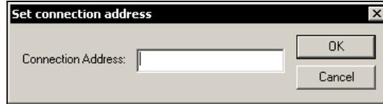
Enter the gas analyzer's IP address or network name in the "Configuration → Set connection address" menu (see also the "Setting TCP/IP Parameters in AO2000" section, page 5).
