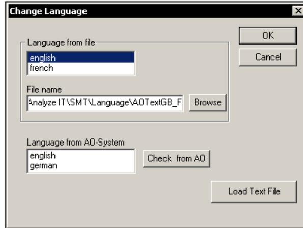
The “Change language” tool is used to load into a gas analyzer a text file containing two languages for the user interface.
