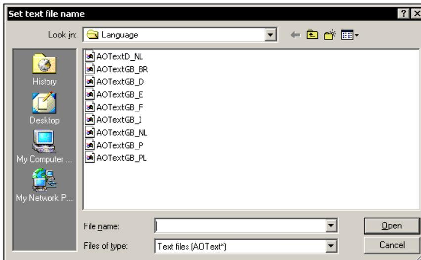
The “Configuration → Set language file” menu is used to enter the name of the text file containing the two gas analyzer user interface languages that will be loaded in the gas analyzer when performing an update.
