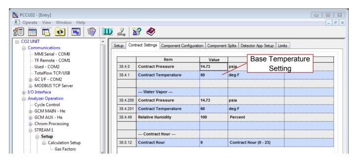
Your product is not affected by this defect, if you are using a base temperature of 60F with GPA-2172, or you are using ISO-6976 for your energy calculations.
