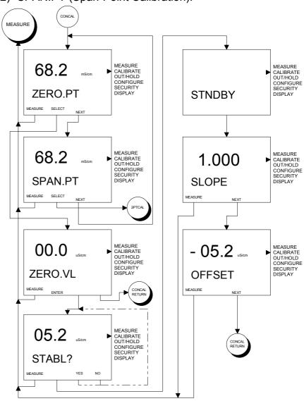
As with the other modes and states of operation, the two calibration procedures can be toggled using the NEXT Smart Key, selected using the SELECT Smart Key, and escaped through the Exit To MEASURE Smart Key.
