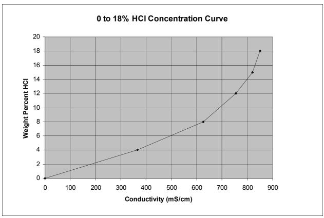
Figure B-3. 0 to 18% HCI Concentration Curve
