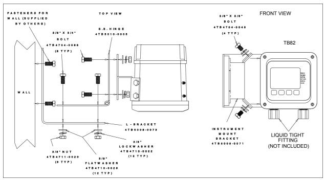
Figure 3-3. Hinge Mount Installation Diagram
