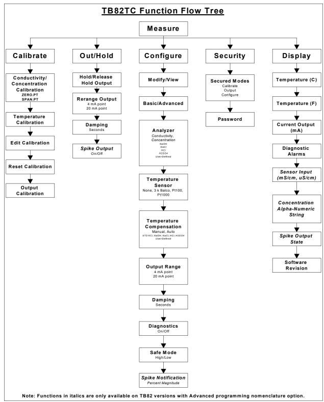
Figure C-1. TB82TC Programming Function Flow Chart.
