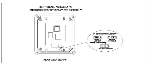
Figure 8-5. Configuration Lockout Jumper Location On Microprocessor/Display PCB Assembly.
