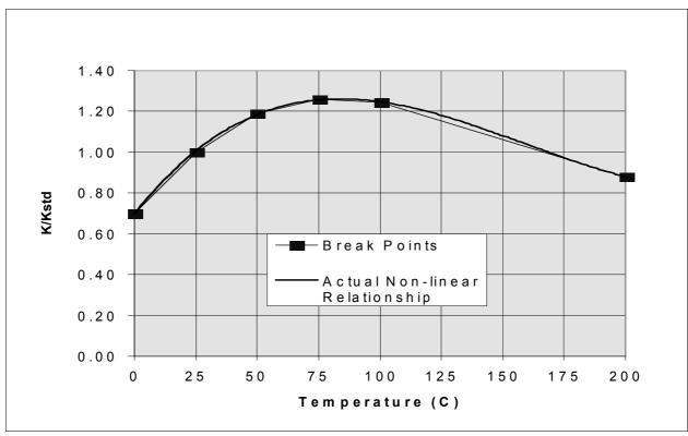
Figure 8-4. User-Defined Temperature Compensation Break Point Determination.
