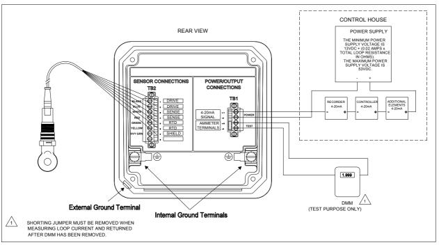
Figure 3-6. Instrument Wiring Diagram
