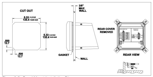
Figure 3-5. Panel Mount Installation Diagram
