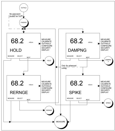
Figure 7-1. Screen Flow Diagrams For Output/Hold States of Operation
