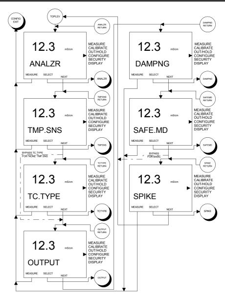
Figure 8-2. Screen Flow Diagram For Modify Configure States of Operation.
