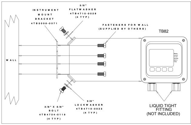
Figure 3-4. Wall Mount Installation Diagram
