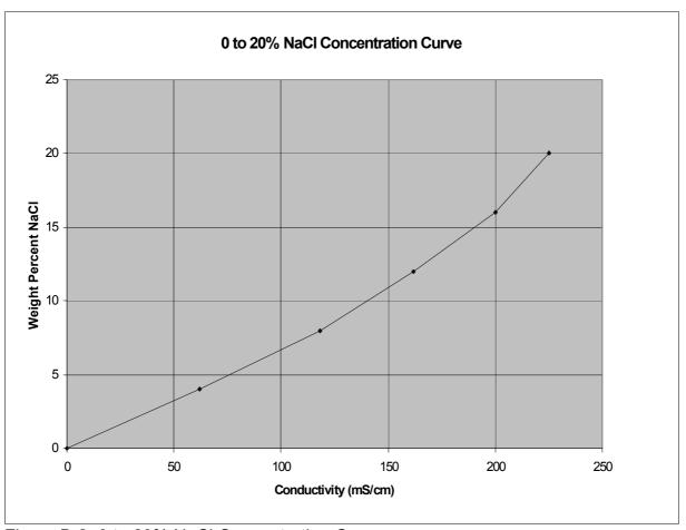
Figure B-2. 0 to 20% NaCl Concentration Curve
