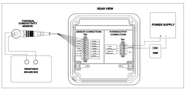
Figure 13-1. Electronic Test Setup.
