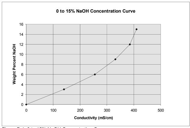
Figure B-1. 0 to 15% NaOH Concentration Curve
