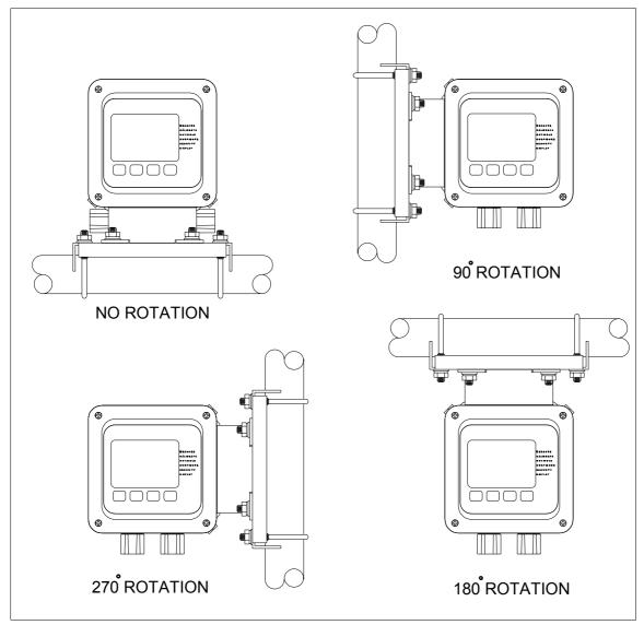
Figure 3-7. Mounting Rotation (Pipe Mount Shown)
