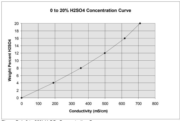
Figure B-4. 0 to 20% H<sub>2</sub>SO<sub>4</sub> Concentration Curve
