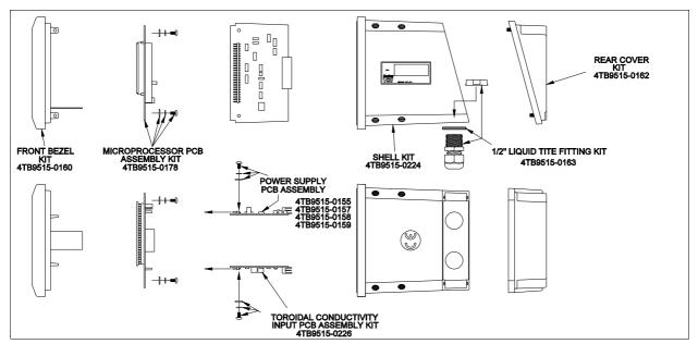
Figure 15-1. TB82 Advantage Series Exploded View Showing Kit Assignments.
