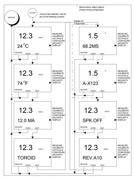
Figure 10-1. Screen Flow Diagrams For Secondary Display States of Operation.
