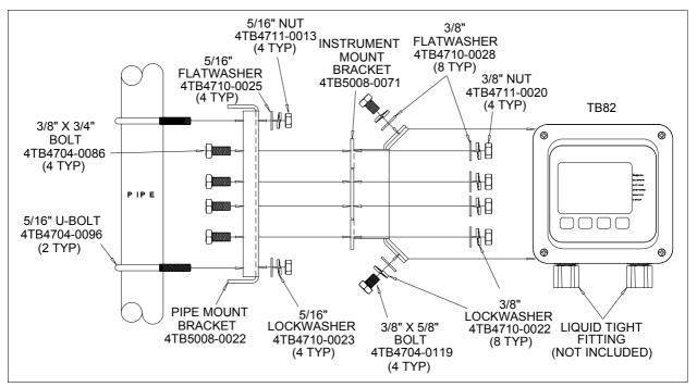
Figure 3-2. Pipe Mount Installation Diagram
