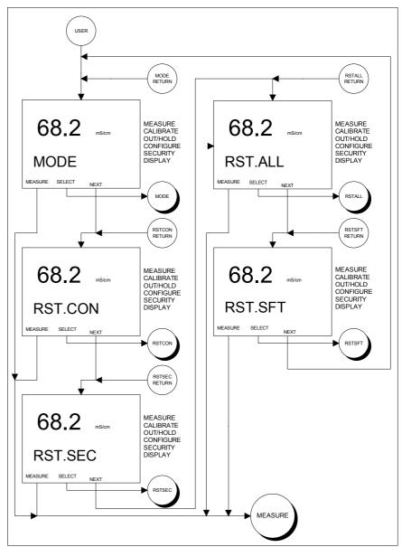
Figure 11-1. Screen Flow Diagram For User States of Operation.
