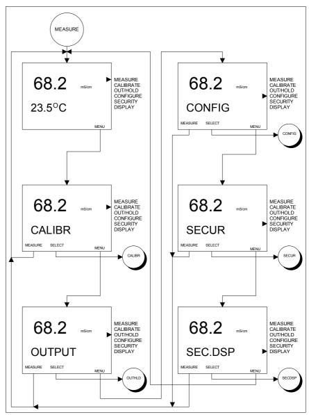
Figure 5-1. Screen Flow Diagrams For Mode of Operation
