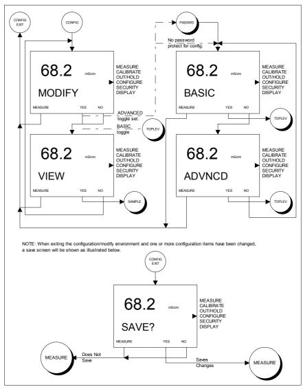
Figure 8-1. Screen Flow Diagram For Modify/View and Basic/Advanced Configure States of Operation.
