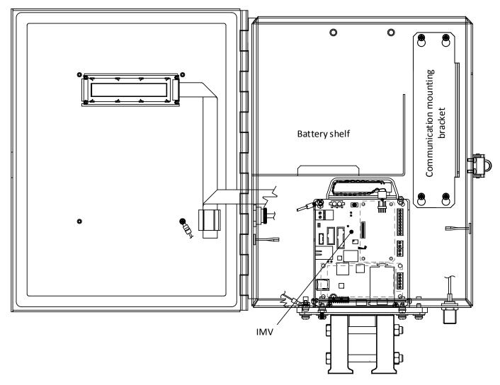
Figure 3:  $\mu$ FLO<sup>G5</sup> enclosure interior
