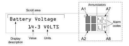
Figure 4: Liquid Crystal Display and annunciators
