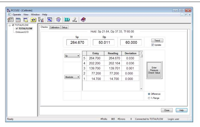
Figure 87: SP calibration pressure checks
