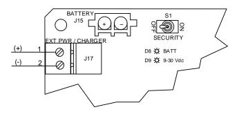
Figure 28: µFLO<sup>G5</sup> power connections and power option selector
