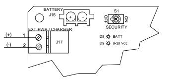
Figure 23: µFLO<sup>G5</sup> power connections and power option selector
