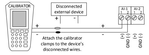
Figure 97: AI calibration equipment
