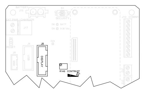
Figure 77: LCD contrast adjustment
