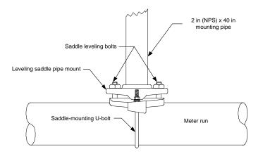
Figure 16: Typical pipe saddle installation
