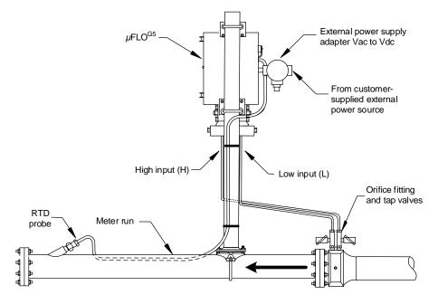
Figure 15: Typical pipe installation
