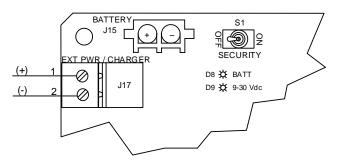
Figure 91: Battery charger and battery connections
