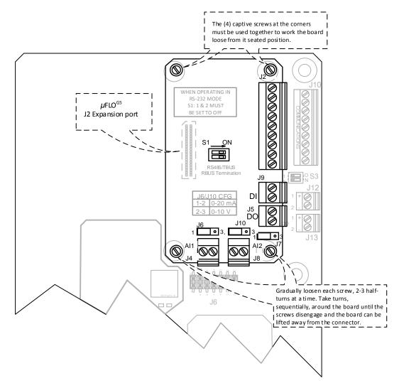
Figure 82: µFLO<sup>G5</sup> board – I/O expansion board removal
