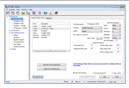
Figure 35: Communications setup screen
