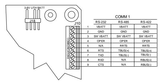
Figure 96: µFLO<sup>G5</sup> Communication Wiring
