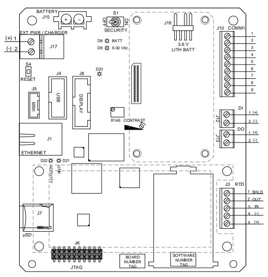
Figure 6: µFLOG5 main electronic board
