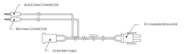
Figure 94: Current measurement troubleshooting cable
