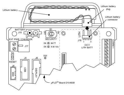
Figure 81: Lithium battery cable and connector
