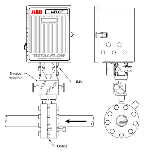
Figure 17: Typical direct mount installation
