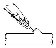
Figure 19: Typical RTD installation
