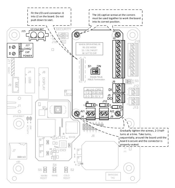
Figure 83: µFLO<sup>G5</sup> board – I/O expansion board replacement
