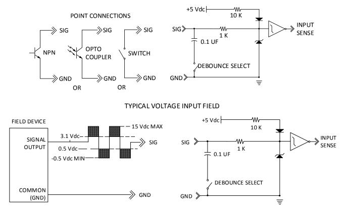
Figure 8: Onboard DI connection examples
