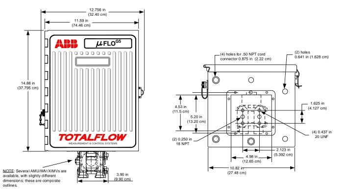
Figure 1: µFLO<sup>G5</sup> enclosure, front and bottom
