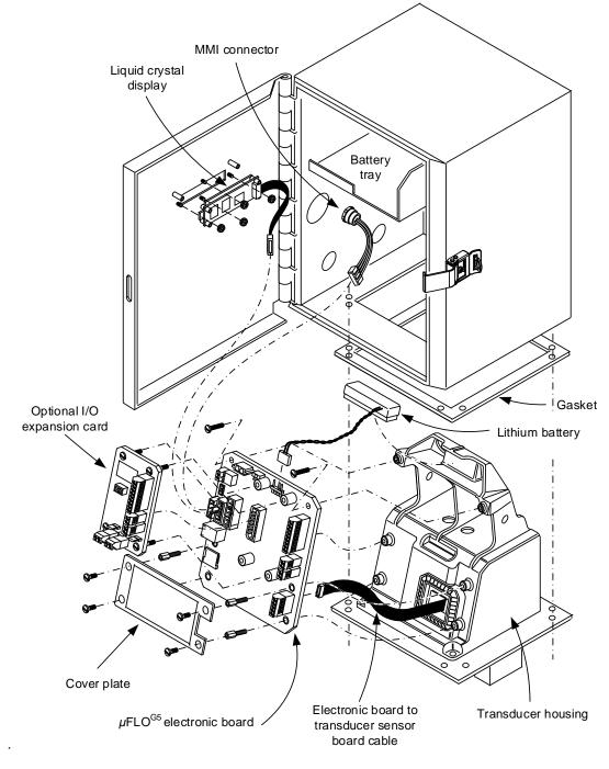
Figure 78: µFLOG5 exploded view
