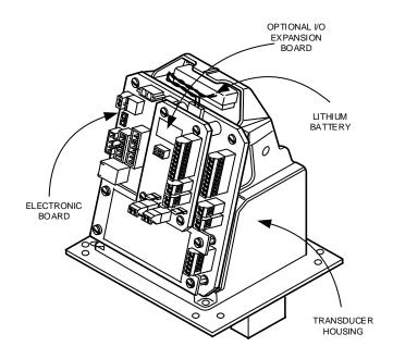
Figure 5: µFLO<sup>G5</sup> IMV assembly (complete)
