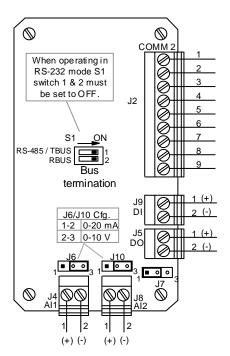
Figure 13: Optional I/O expansion board
