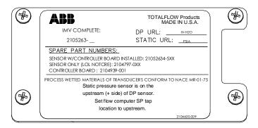
Figure 84: Cover plate with transducer information
