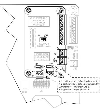
Figure 98: Analog Input mode selection
