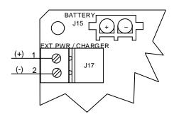
Figure 76: µFLO<sup>G5</sup> electronic board power connections
