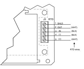
Figure 21: RTD sensor wiring to  $\mu$ FLO<sup>G5</sup> electronic board
