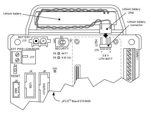
Figure 25: Lithium battery and connector
