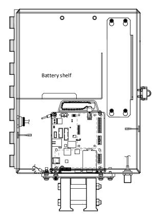
Figure 24: µFLO<sup>G5</sup> enclosure inside view
