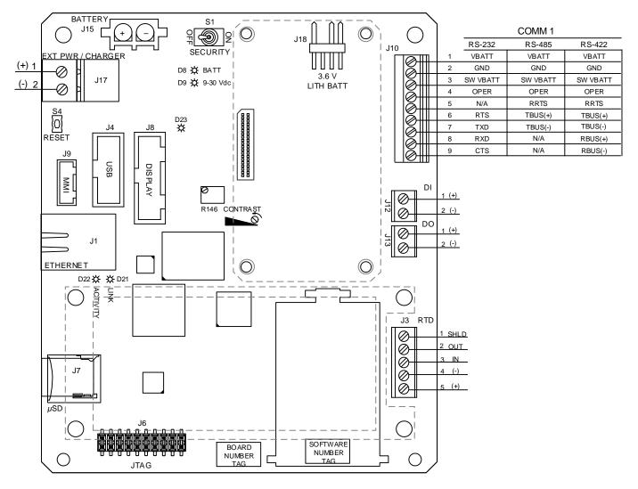
Figure 93: µFLO<sup>G5</sup> board field wiring connections
