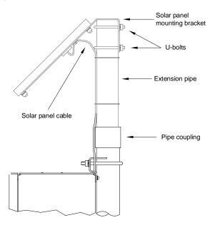
Figure 22: Solar panel installation
