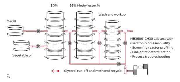
The MB3600-CH30 laboratory FT-NIR analyzer is designed and configured for routine biodiesel analysis and easy calibration modeling and method preparation. It includes all the hardware, software and accessories required for both biodiesel measurement and chemometrics method development.
