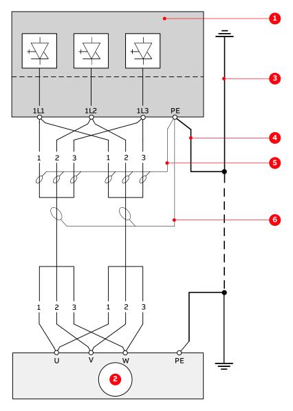
Figure 6-4 Grounding the drive and the motor (single-point bonding)
