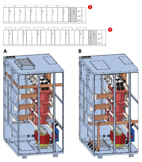
Figure 3-17 Motor terminal section of frame size 3 and 4: top entry (A) and bottom entry (B)
