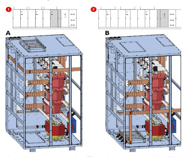
Figure 3-16 Motor terminal section of frame size 1 and 2: top entry (A) and bottom entry (B)
