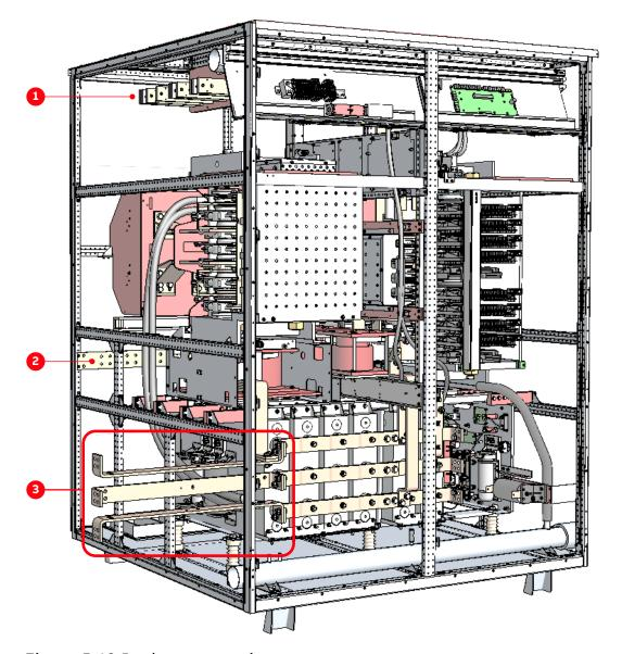
Figure 5-10 Busbar connections
