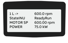
2. To select a line where the actual signal is to be displayed, press the slow navigation keys.
