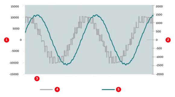
Figure 3-3 Principle of 9-level topology
