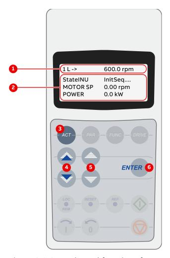
Figure 9-2 Control panel functions for Actual signals mode
