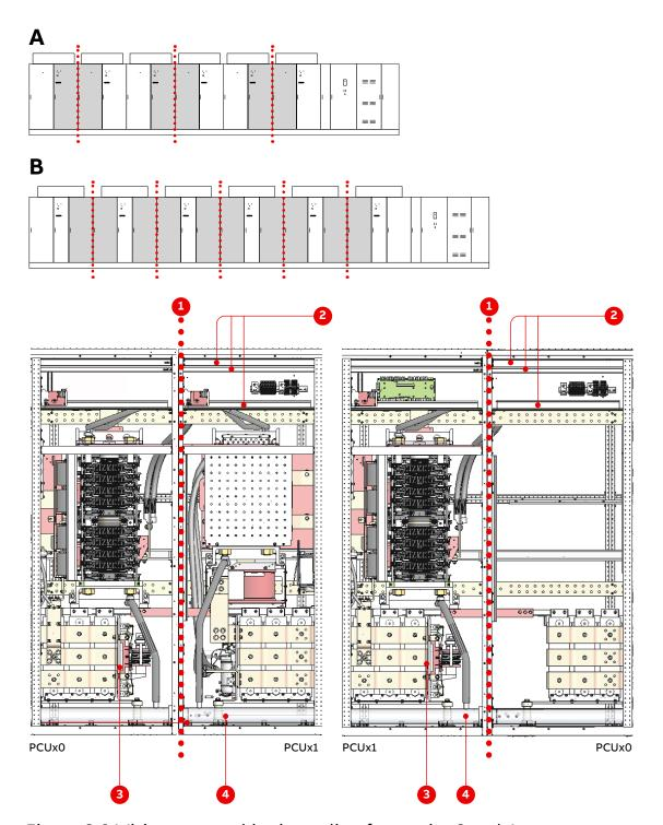
Figure 6-8 Wiring across shipping splits, frame size 3 and 4
