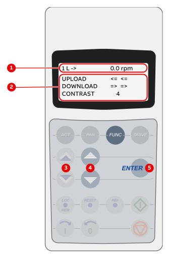
Figure 9-4 Control panel functions for Functions mode
