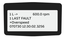
**3.** To display a specific fault, press the slow navigation keys. The up key selects the previous, the down key the next fault.
