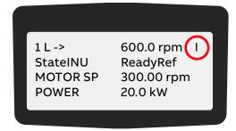
As long as the stop sequence is in progress, you can always restart the drive by pressing the START key.
