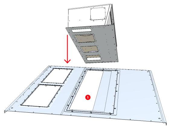
2. Slowly lower the cooling unit onto the cabinet roof.
