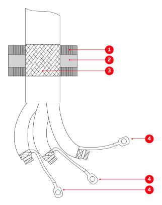
Figure 6-21 Preparing control cables for sealing modules
