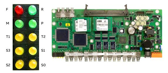
Figure 10-3 LEDs of AMC circuit board
