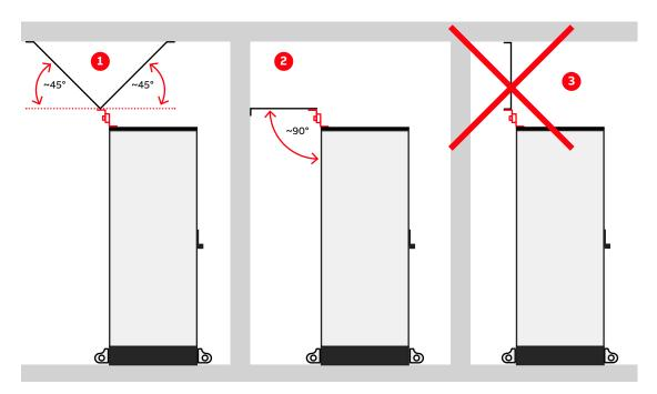
Figure 5-9 Recommended ceiling and wall fixings
