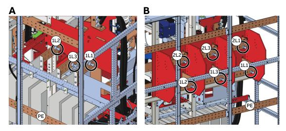
Figure 3-27 Connection studs for the 4-way grounding set in an 18-pulse ACS5000WPCU (A) and a 36-pulse ACS5000W PCU (B)
