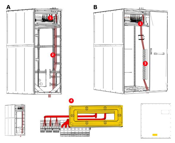
Figure 6-23 Cable routing in WCU800 (A) and WCU1400 (B) cabinets
