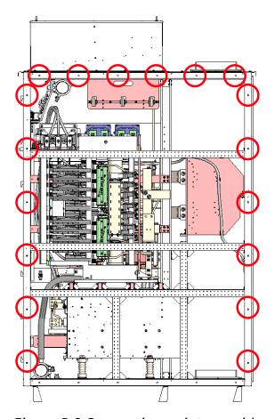
Figure 5-2 Connection points on side of transport units (PCU example)
