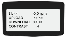
**2.** To select the contrast adjustment function, press the slow navigation keys until the **blinking** cursor reaches the CONTRAST line.
