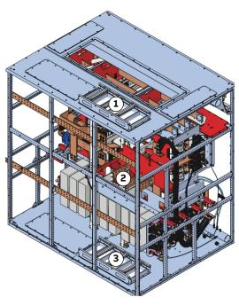
Figure 6-17 PCU 18-pulse top and bottom entry (back view)
