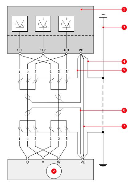
Figure 6-3 Grounding the drive and the motor (multi-point bonding)
