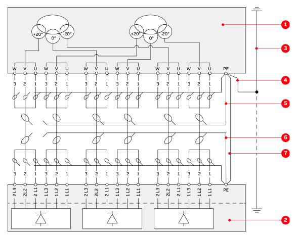
Figure 6-2 Grounding the transformer and a 36-pulse drive (in PCU)
