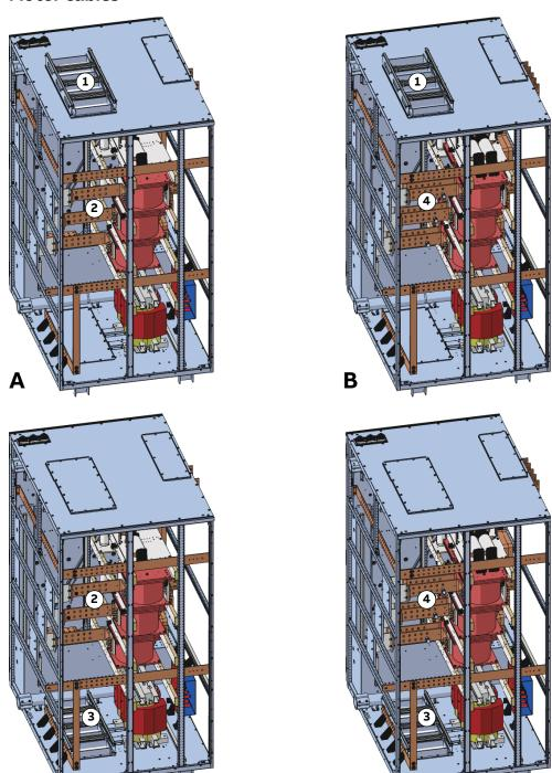
Figure 6-18 COU cable terminals, top and bottom entry (back view) - frame sizes 1 and 2 (A) and 3 and 4 (B)  $^{\circ}$
