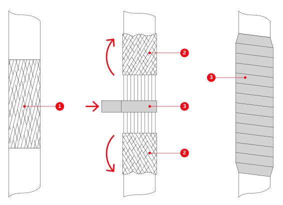
Figure 6-20 Preparing control cables for EMC plates
