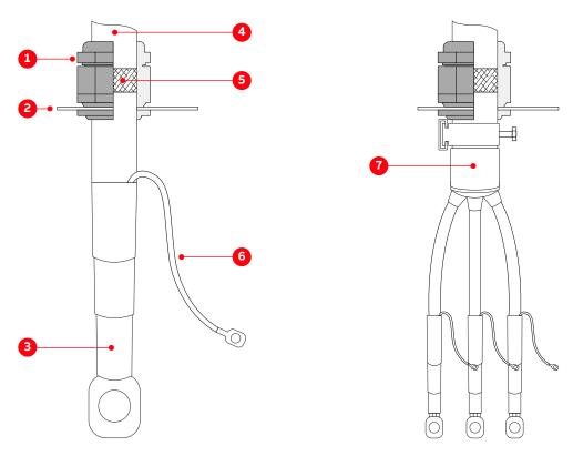
Figure 6-14 Preparing power cables for cable glands
