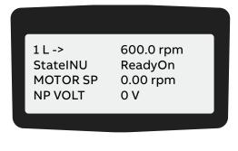
7. To cancel the selection and keep the original selection, press any of the mode selection keys. The selected keypad mode is entered.
