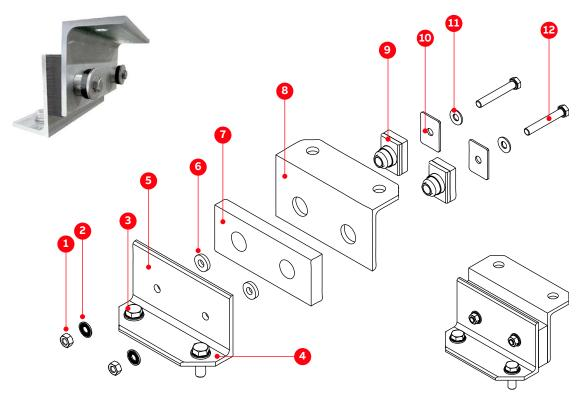
Figure 5-8 Roof attachment
