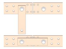
Figure 5-12 PE ground busbar connection
