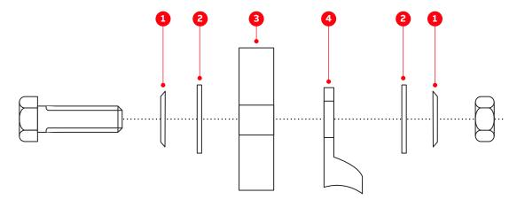
Figure 6-19 Bolted busbar connection
