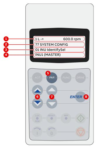
Figure 9-3 Control panel functions for Parameters mode
