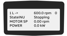
When the motor has reached zero speed, the status line displays ReadyRun.
