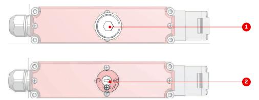
2. Turn out the locking screw (1) until the release dial can be turned.
