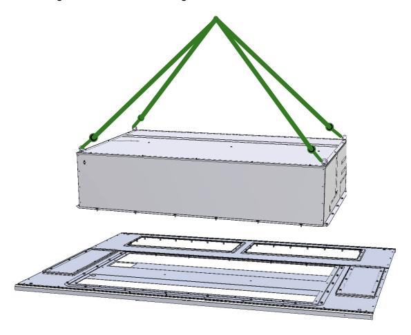
Figure 5-5 Lifting a cooling unit (example with IP54 unit)
