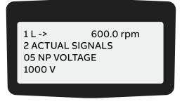
**6.** To confirm the selection and to return to the actual signals display, press the ENTER key.
