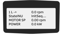
After another few seconds, the display changes to the actual signals display. The status line of the display alternates between DCGndNOpen and NotReadyOn.
