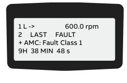
4. To clear the fault memory, press the RESET key.
