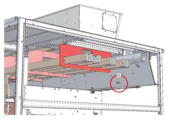
Figure 5-6 Cable duct openings (example with 1700 mm PCU)
