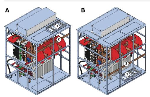
Figure 6-6 PE ground busbar in a PCU frame size 1 (A) and frame size 2 (B)
