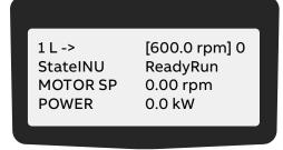
6. To start the motor, press the START key.
