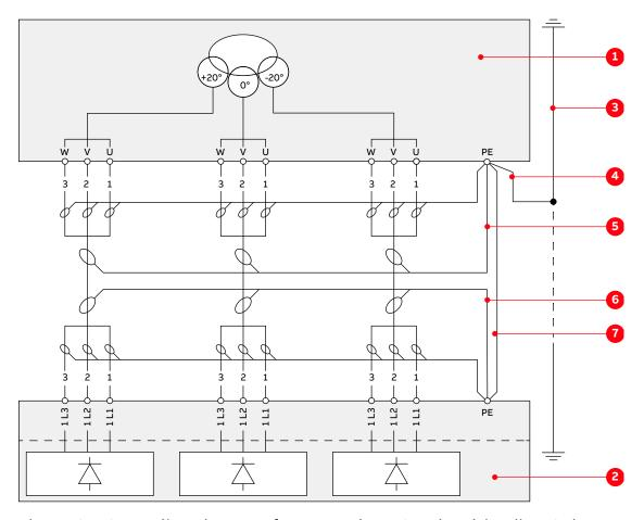
Figure 6-1 Grounding the transformer and an 18-pulse drive (in PCU)
