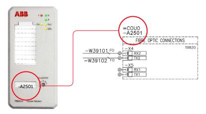
Figure 10-1 Device identification
