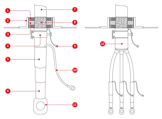
Figure 6-15 Preparing power cables for sealing modules
