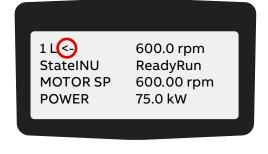
If you change the direction while the motor is running, the motor automatically ramps down to zero speed and reaccelerates in the opposite direction to the preset speed. The arrow changes at zero speed.
