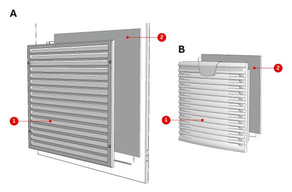
Figure 10-8 Filter mat replacement for PCU (A) and WCU (B)
