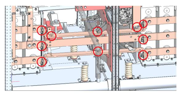
Figure 5-13 DC busbar connection
