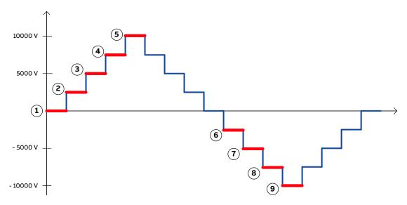
Figure 3-2 Switching levels
