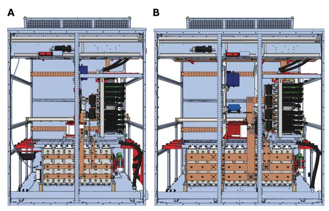
Figure 3-10 Secondary PCU, 1700 mm (A) and 2100 mm (B)
