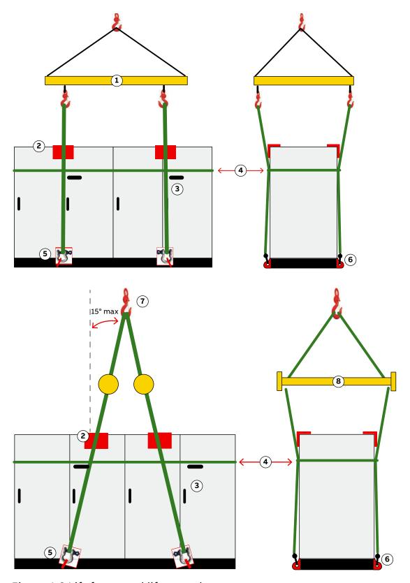
Figure 4-2 Lift frame and lift spreader
