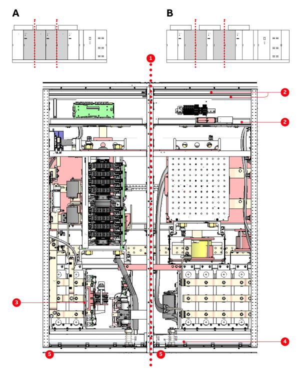
Figure 6-7 Wiring across shipping splits, frame size 1 (A) and 2 (B)
