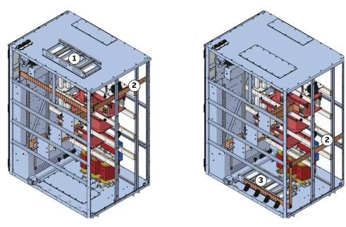
Figure 6-5 PE ground busbar in a COU
