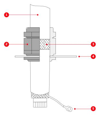
Figure 6-22 Preparing control cables for cable glands
