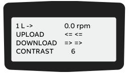
**6.** To cancel the setting and keep the original setting, press any of the mode selection keys. The selected keypad mode is entered.
