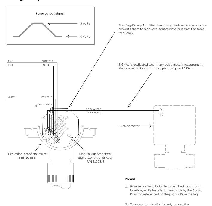
1. The preamp is DC coupled and can sense differential signals down to 0 Hz. However, inductive pickups do not generate signals this low since they are
