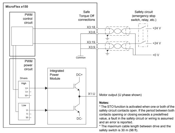
**WARNING!** The STO function does not disconnect the voltage of the main and auxiliary circuits from the drive. Therefore maintenance work on electrical parts of the drive or the motor can only be carried out after isolating the drive system from the main supply. If the drive was connected to the input power, wait for 5 minutes after disconnecting the input power.
