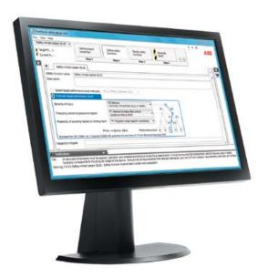
The functional safety design tool (FSDT-01), helps you design and calculate safety integrity levels (SIL)/performance levels (PL) for safety functions and generate safety calculation reports.
