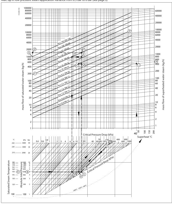
Steam valve sizing is based on 40 % of the absolute steam pressure (immediately upstream of the valve), being dropped across the valve when fully open. At this condition the steam is travelling at or close to its critical velocity
