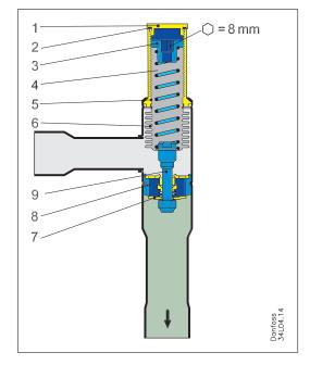
Crankcase pressure regulator type KVL opens on a fall in pressure on the outlet side, i.e. when the suction pressure falls below the set value. Type KVL regulates on outlet pressure only. Pressure variations on the inlet side of the regulator do not affect the degree of opening as the valve is equipped with equalization bellows (6). The bellows has an effective area corresponding to that of the valve seat neutralizing any affect to the setting.
