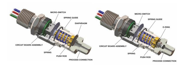
Cutaway view of switch assembly with welded SS diaphragm
