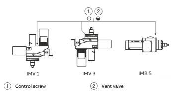
Figure 7: Mounting positions RSD50 / RSD100
