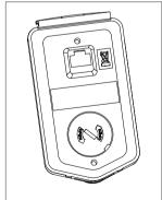
To reinstall the control panel, put the bottom of the container in position (1a), press the retaining clip at the top (1b) and push the control panel in at the top edge (1c).
