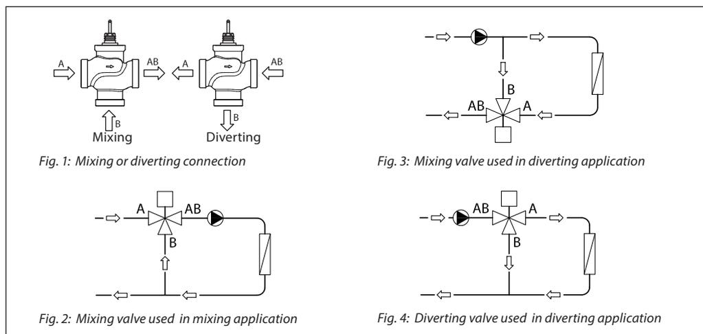
Mixing or diverting connection
