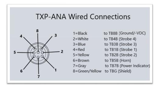
Figure 3-4 – Cable Pinout wiring
