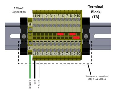
Figure 3-5 – Terminal Block wiring
