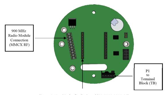
Figure 4-12 - Display/Radio Board (83-8008-0000-00)
