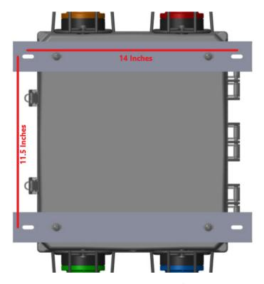
Figure 3-1 – Mounting Holes
