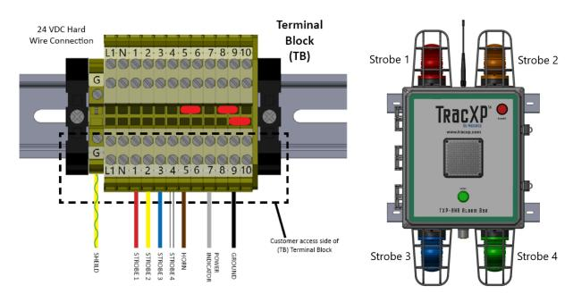
Figure 3-2 – Terminal Block connections
