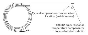
Figure 3 TBX587 temperature compensator location
