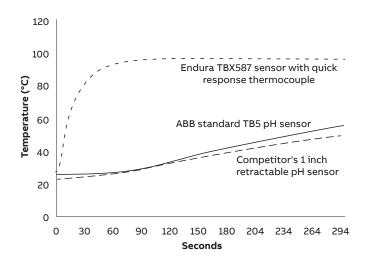
Figure 2 TBX587 thermocouple response time
