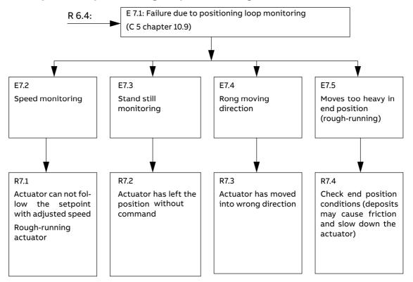
Figure 44: Failure due to response of positioning loop monitoring
