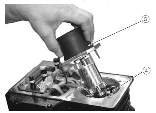
Figure 13: Brake body with rotor
