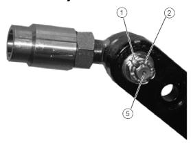
Figure 7: Ball-and-socket-joint
