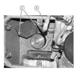
Figure 33: Free access to sensor of PME120-AI
