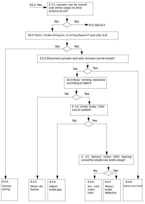
Figure 39: Failures at brake, fuse or wiring
