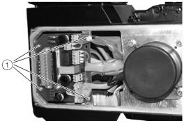
Figure 32: Removal of connection pcb at PME120-AI
