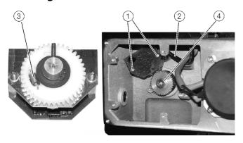
Figure 34: Position sensor / Mounting position (example shows PME120-AN)
