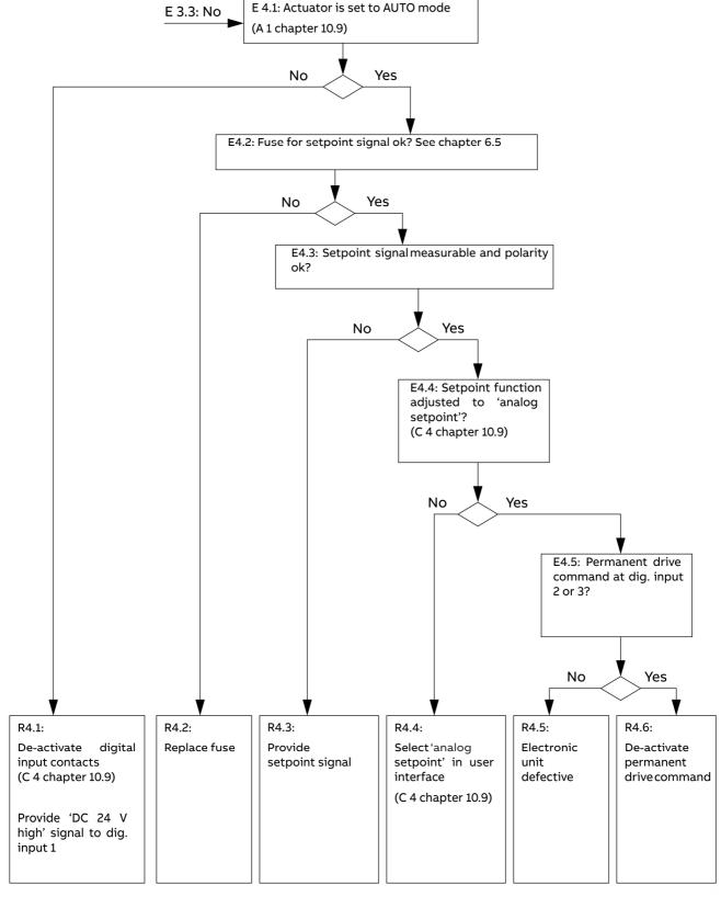
Figure 41: Input configuration
