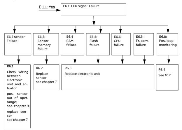
Figure 43: Failure Diagram
