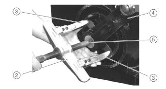
Figure 6: Use of draw-off tool for lever removal
