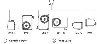
Figure 4: Permissible mounting positions
