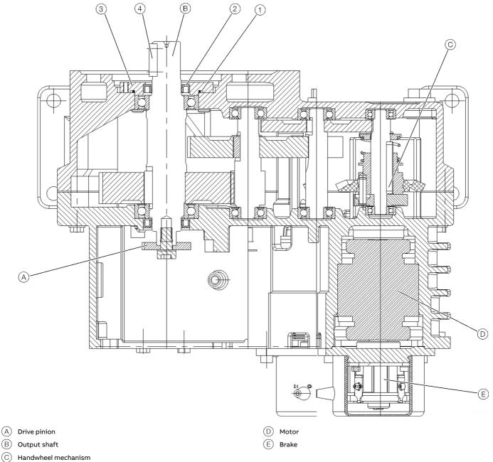
Figure 9: Sectional view of PME120
