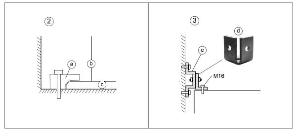
2. Clamping the cabinet to the floor at the back
