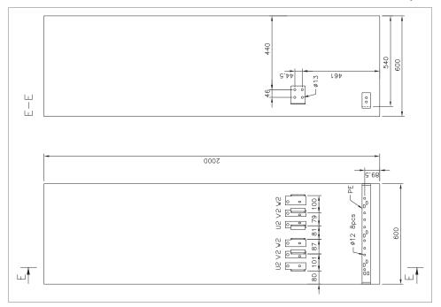
Inverter module cubicle with two R8i modules, top cable exit (+H353)
