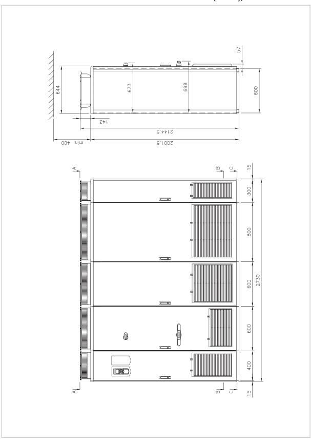
Frame 2×D8T + 3×R8i with common motor terminal cubicle (+H359), 2/2
