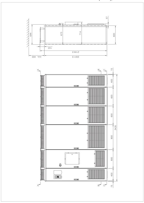
Frame 3×D8T + 4×R8i with common motor terminal cubicle (+H359), 2/2
