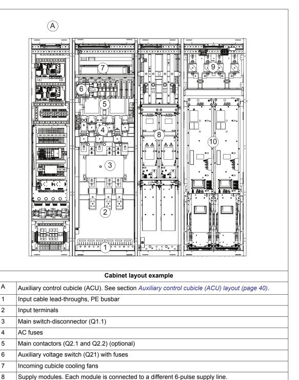
Inverter modules. The output terminals are located behind each module. Each module must be individually connected to the motor using separate cables unless the drive is equipped with option +H359 (common motor terminal cubicle), +H366 (common output terminals) or +E206 (sine filters).
