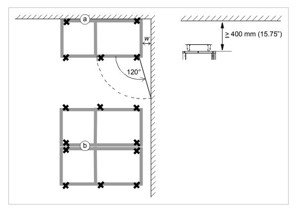
**Note 1:** Any height adjustment must be done before fastening the units or shipping splits together. Height adjustment can be done by using metal shims between the cabinet bottom and floor.
