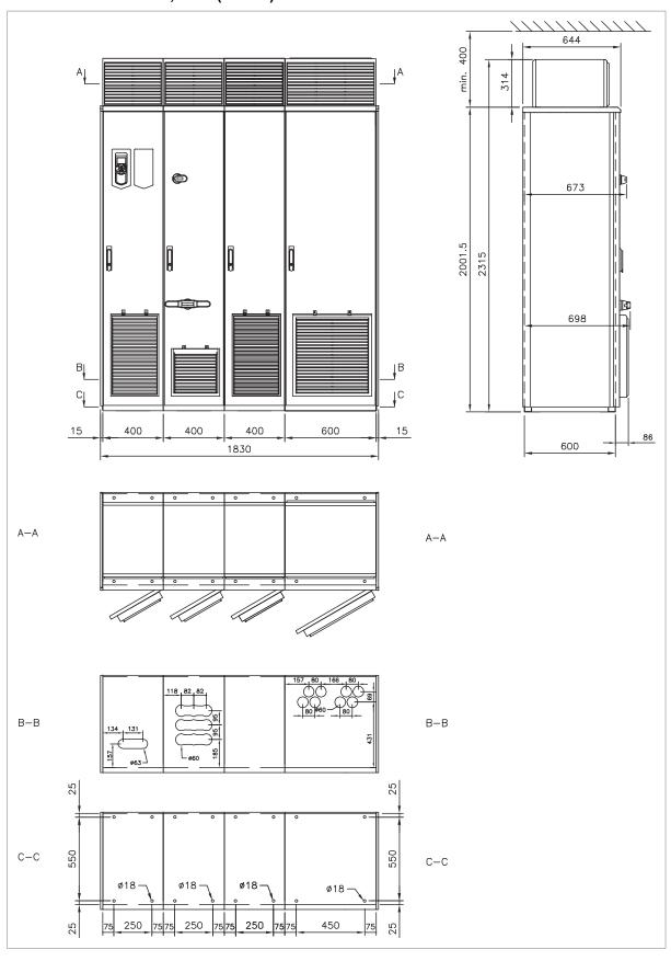
Frame 1×D8T + 2×R8i with common motor terminal cubicle (+H359), 1/2
