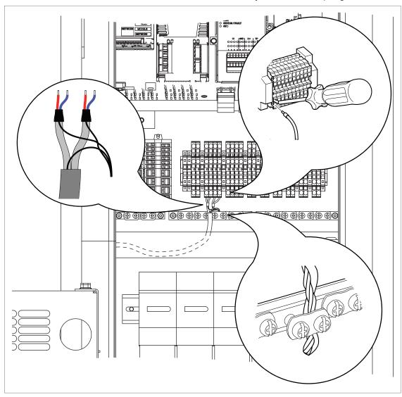
At the other end of the cable, leave the shields unconnected or ground them indirectly via a high-frequency capacitor with a few nanofarads, eg. 3.3 nF / 630 V. The shield can also be grounded directly at both ends if they are in the same ground line with no significant voltage drop between the end points.
