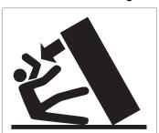
• Be careful when handling a tall module. The module overturns easily because it is heavy and has a high center of gravity. Whenever possible, secure the module with chains. Do not leave an unsupported module unattended especially on a sloping floor.
