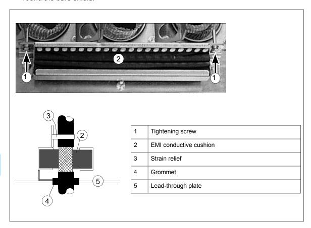
**Note 1:** Keep the shields continuous as close to the connection terminals as possible. Secure the cables mechanically at the lead-through strain relief.
