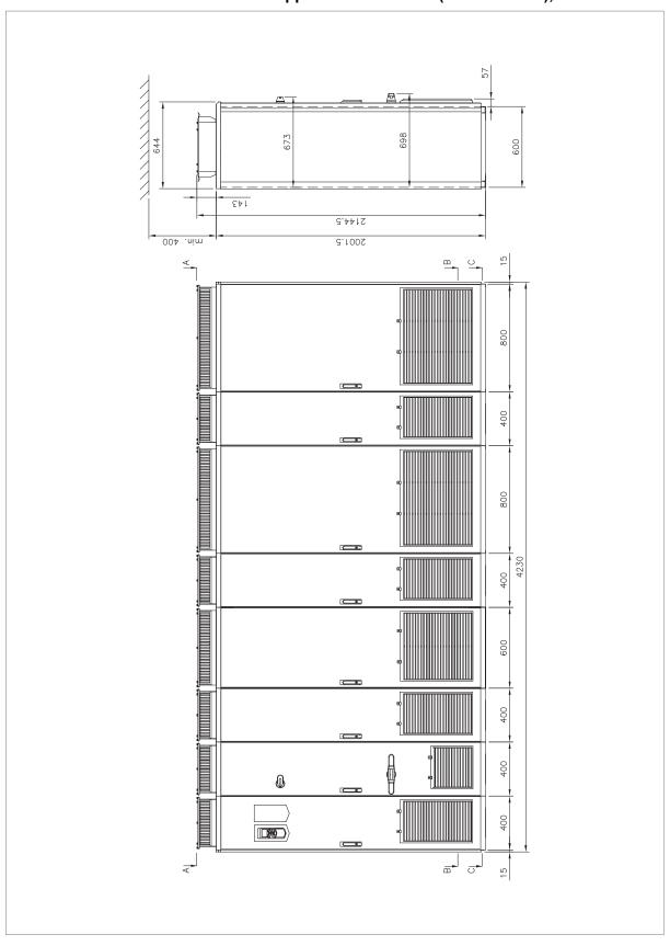
Frame 1×D8T + 2×R8i with brake choppers and resistors (+D150 +D151), 2/2
