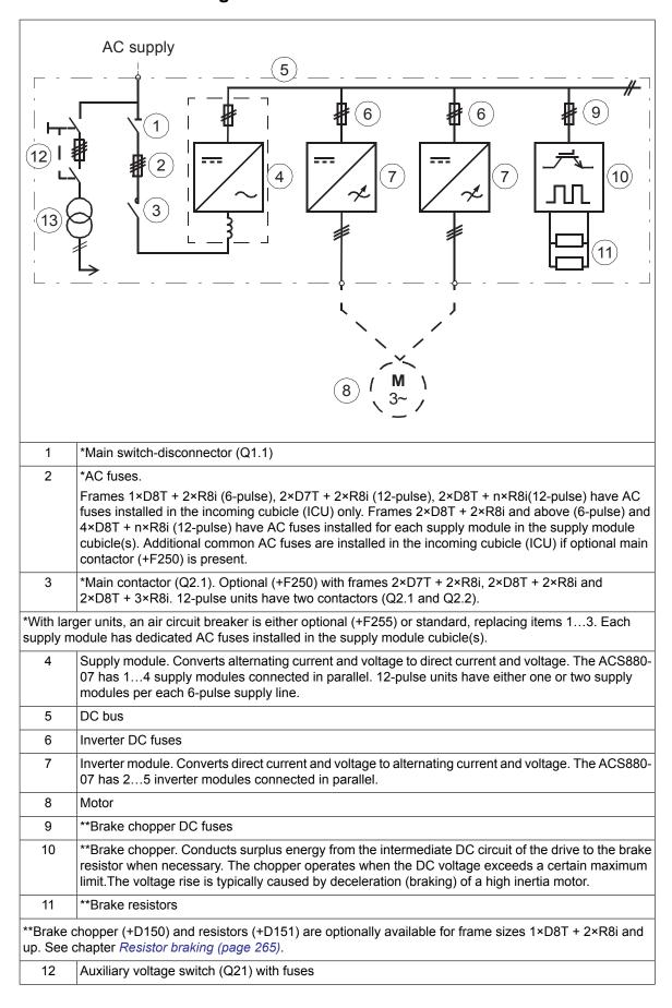
Auxiliary voltage transformers (T21, T101, T111). T21 is standard; T101 and T111 are added whenever required by the options ordered.
