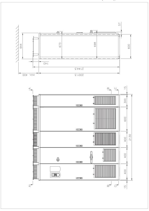
Frame 1×D8T + 2×R8i with common motor terminal cubicle (+H359), 2/2
