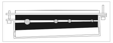
6. If more than one cable go through a grommet, seal the grommet by applying Loctite 5221 (catalogue number 25551) inside the grommet.
