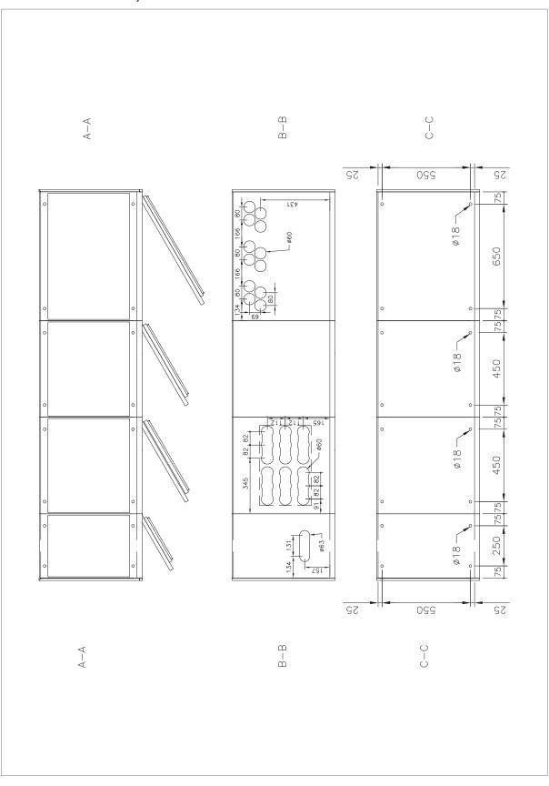
Frame 2×D8T + 3×R8i with common motor terminal cubicle (+H359), 1/2
