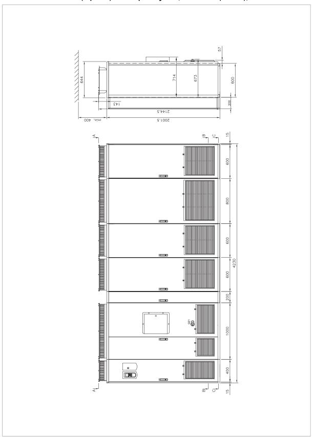
Frame 4×D8T + 5×R8i (6-pulse) with top entry/exit, UL Listed (+C129), 2/2
