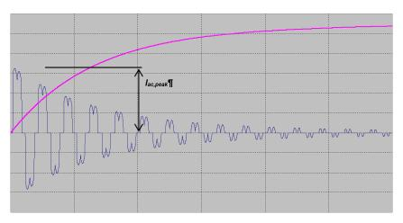
It is essential to check that the AC supply side components (fuses, contactors, etc.) can withstand the peak current at start up. The peak current  $I_{ac,peak}$  is calculated as follows:
