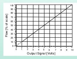
This chart shows linear characteristics of the F-series flow monitor with a signal output of 1-10 volts. Characteristics would be similar for 5.6-20 mA units.
